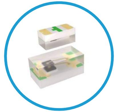
VAOL-S4 Series is a SMD LED with high intensity light output and a clear non-diffused lens
