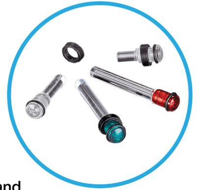
Clear Acrylic UL94-HB Light Pipe. Available in different length and colors and fit into 0.171" (4.34mm) panel hole diameter with a panel thickness of 0.031" (0.8mm) to 0.094" (2.39mm)
