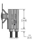
Wire Leads: No. 22 AWG (105°C) 4.40"/4.80" long, stripped .430"/.570" Lens: Polycarbonate Housing: Nylon
