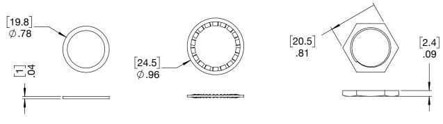
Washer: EPDM Lock Washer: SPCC Nickel Plated Hex Nut: Brass Nickel Plated
