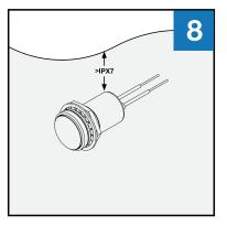
Protected against the effects of permanent submersion in water. (Up to 3.9 meter)
