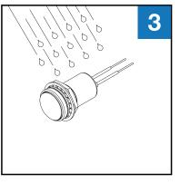
Protected against water spray at any angle up to 60° from the vertical.
