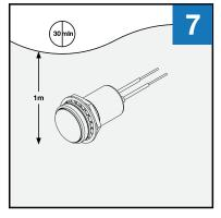
Protected against the effects of temporary submersion in water (30 min at 1 meter)
