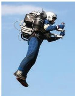
The jetpack is designed to automatically communicate changes in fuel load to the pilot during takeoff and flight. The advanced jetpack pilot warning display quickly and accurately provides all necessary information to the pilot including exhaust gas temperature, battery voltage, electronic control unit, and calibration.
