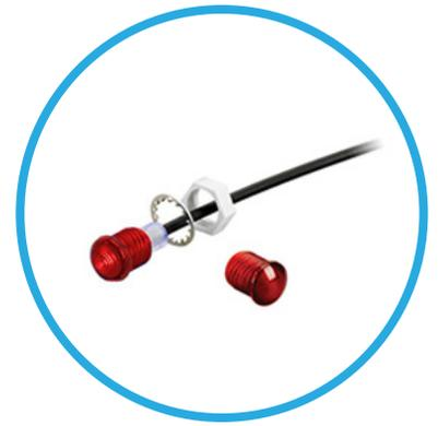
Easy panel installation – insert lens through panel hole from and from the back slide slip the lock washer onto lens barrel. While holding lens, twist on retaining ring one revolution until secure
