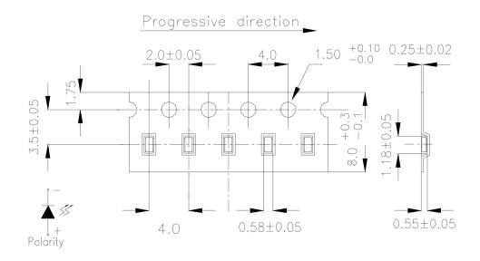
**Note:** The tolerance unless mentioned is  $\pm$  0.1mm, Unit=mm
