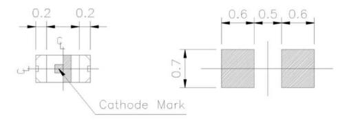
**Note:** The tolerance unless mentioned is  $\pm$  0.1mm, Unit=mm
