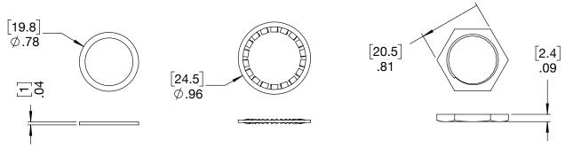
Washer: EPDM Lock Washer: SPCC Nickel Plated Hex Nut: Brass Nickel Plated
