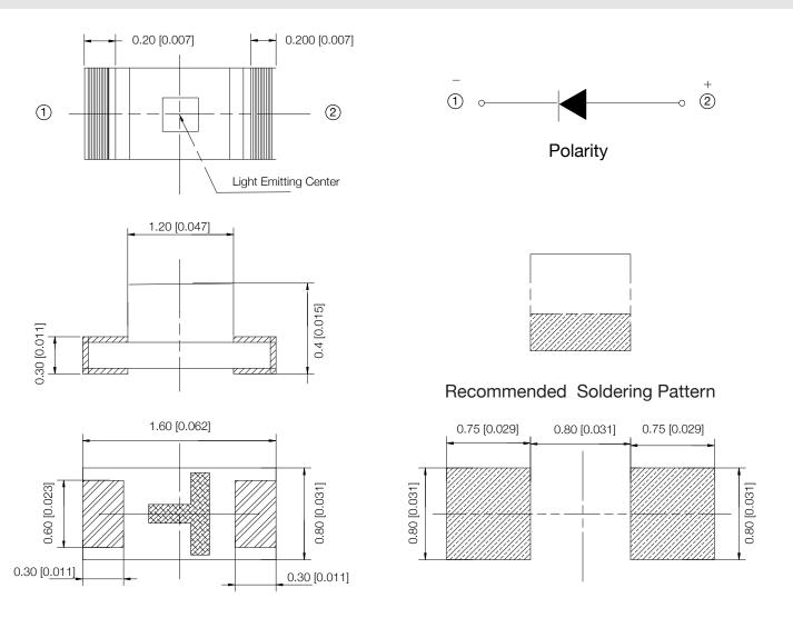
Note: The tolerance unless mentioned is ± 0.1mm [0.005 in]; Unit=mm [in]
