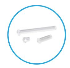
2.5mm round Light Pipe mount securely to display panel providing 160° viewing angle. Available in different lengths fit into 0.102" (2.59mm) panel hole diameter on 3/16" centers.
