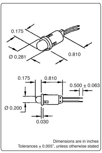
LED Indicator Light 2 to 24 Volts DC Clear or Diffused LED 1/4" Mounting Hole
