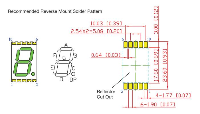
$\label{eq:Dimensions} \mbox{Dimensions in millimeters [inches]} \\ \mbox{Tolerance is $\pm 0.25 mm [.01"] unless otherwise noted}$
