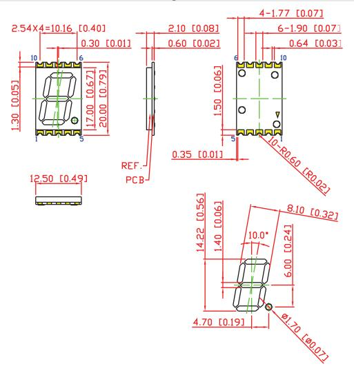
Dimensions in millimeters [inches] Tolerance is  $\pm 0.25$ mm [.01"] unless otherwise noted
