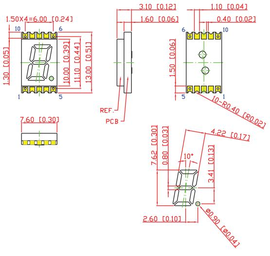
Dimensions in millimeters [inches] Tolerance is  $\pm 0.25$ mm [.01"] unless othewise noted
