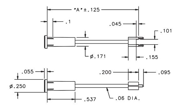
Front to press fit into 0.187"+/-0.02 Dia. hole circuit board mounting pattern for use with CMDA19 Series LED
