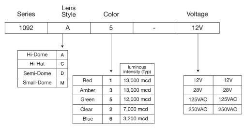
Example: 1092A5-12V 1092 with Hi-Dome lens - Green LED and 12 Volts
